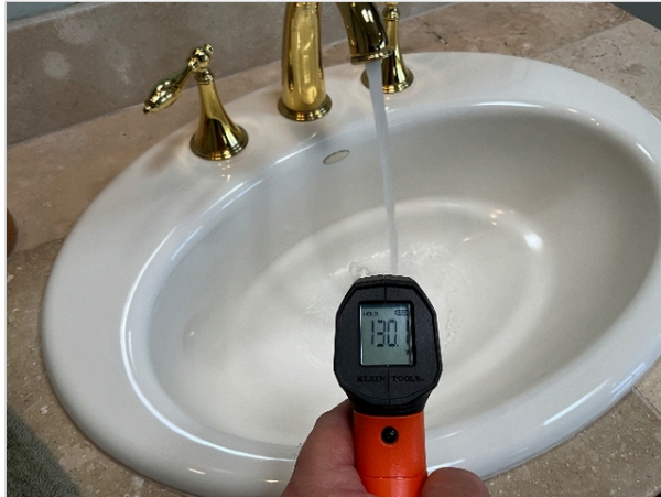
Measured water temperature
